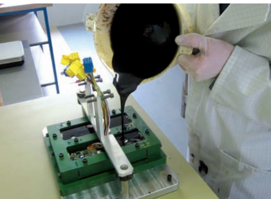
>>> Potting - Encapsulation of electronic assembly
